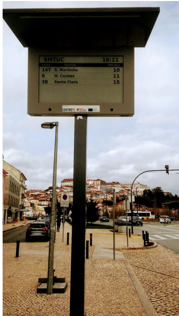
Figure 20 Real time information schedules on an outdoor e-paper technology and solar energy panel
