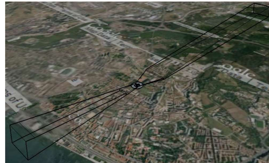
Figure 10: Airship surface-level and obstacle limitations surfaces
