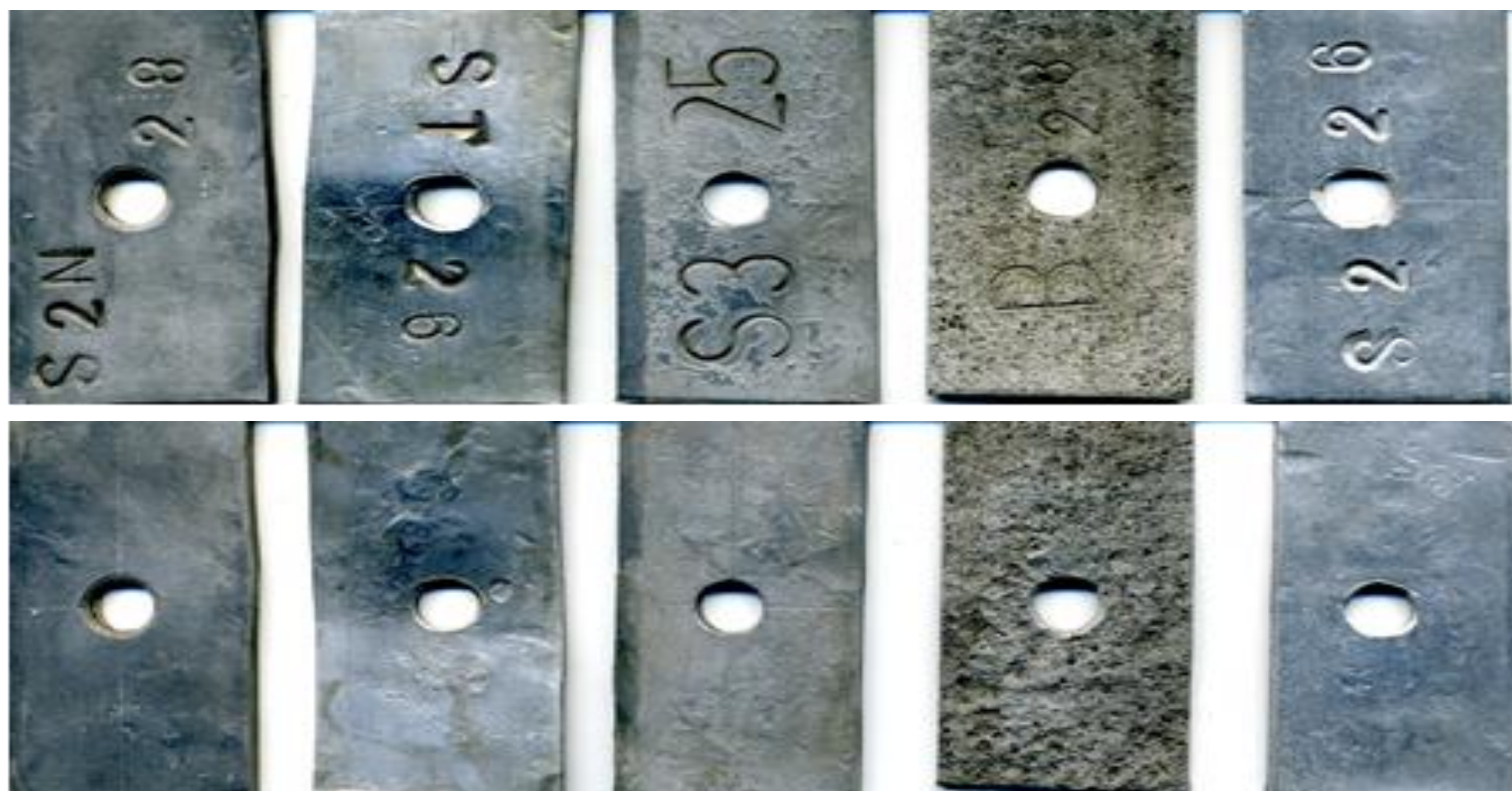
Coupons cleaned after exposition to corrosive factors
