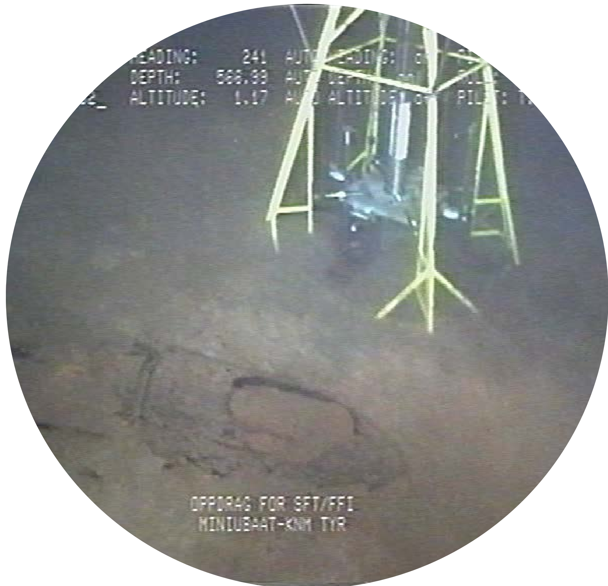
Corroded bomb shell and sediment sampler in Skagerrak in 2002 (Photo:FFI)
