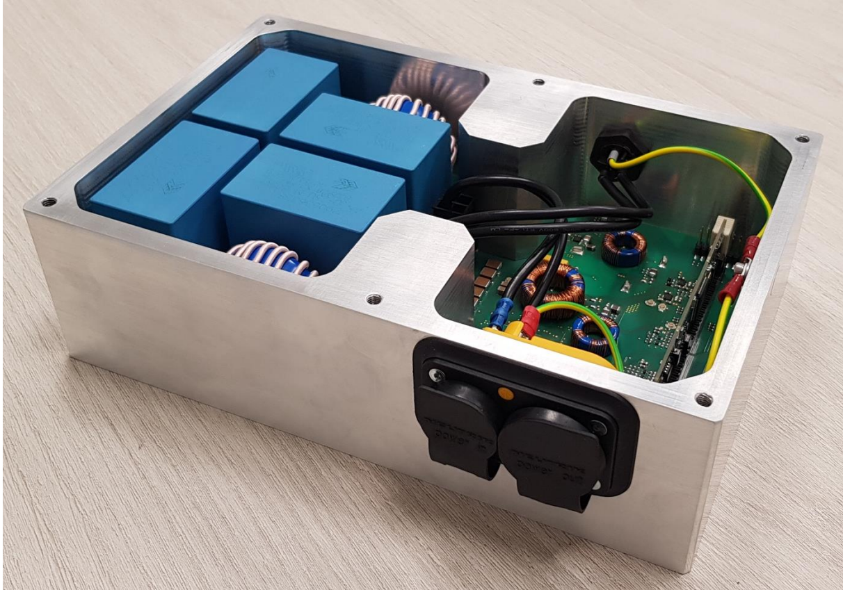
Figure 2.5: Picture of the realized single phase DC/DC converter with the control board, the connectors, the internal flyback and buck converters on the right and the passive components on the left hand.
