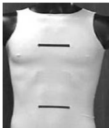
Knitted system for the acquisition of abdominal and thoracic respiratory activity https://www.researchgate.net/publication/224703744_Sensing_Fabrics_for_Monitoring_Physiological_and_Biomechanical_Variables_E-textile_solutions/figures?lo=1
