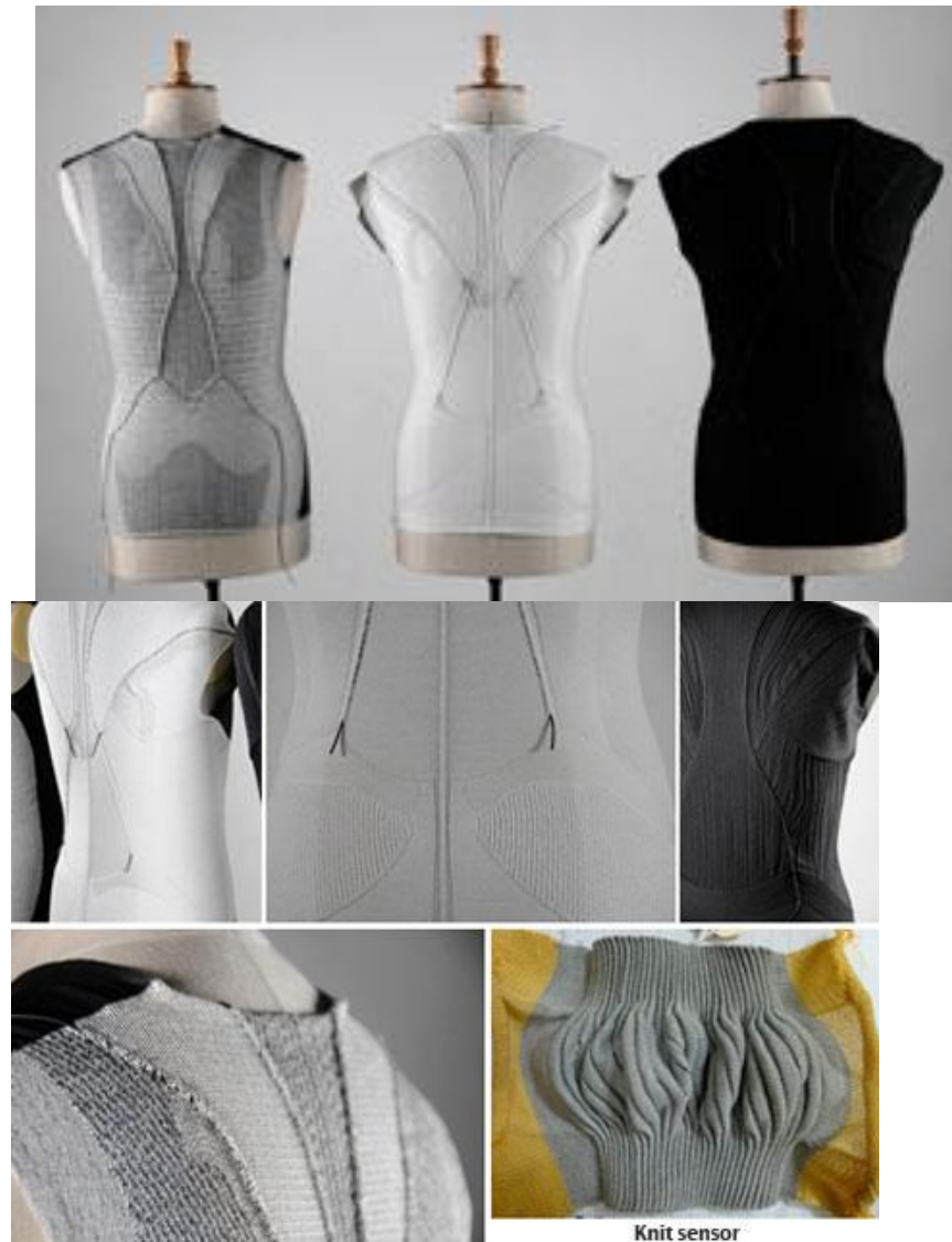
8.fig. Knitted sensors - tensile sensors, breathing control clothing [29][32][33][34][35]
