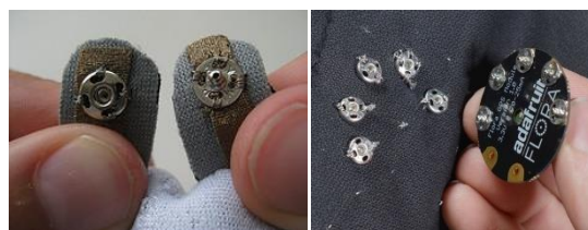
22.fig. Clamping of the electrically conductive chain with push buttons a) Pushbutton and conductive cloth b) ‘Adafruit’ module
