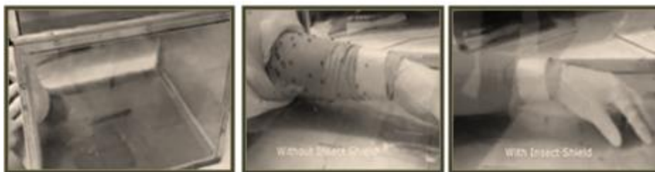
42.att. Arm-in-Cage test precess [124]
