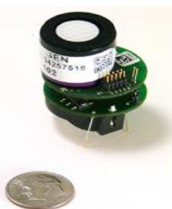
37.fig. Texas Instruments gas Sensor Platform with bluetooth Low Energy Evaluation Module [111]
