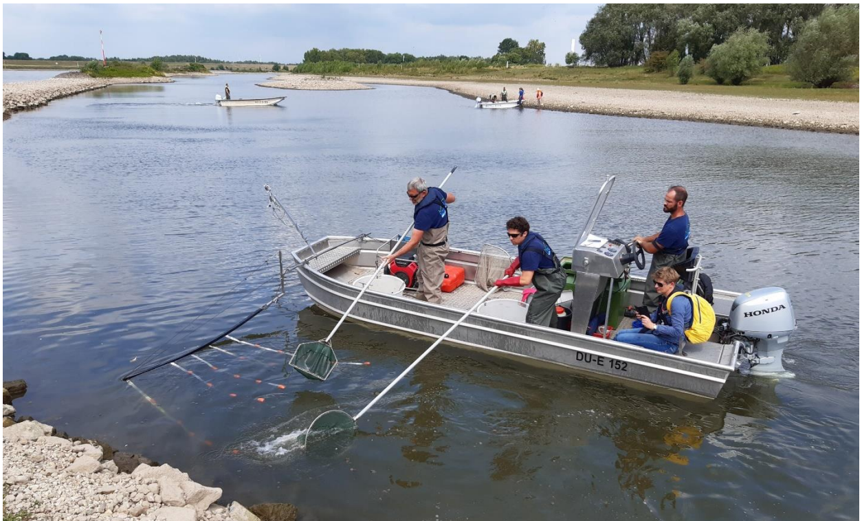
Figure 4 Strip anode electrofishing as applied by the German team from LimnoPlan.
