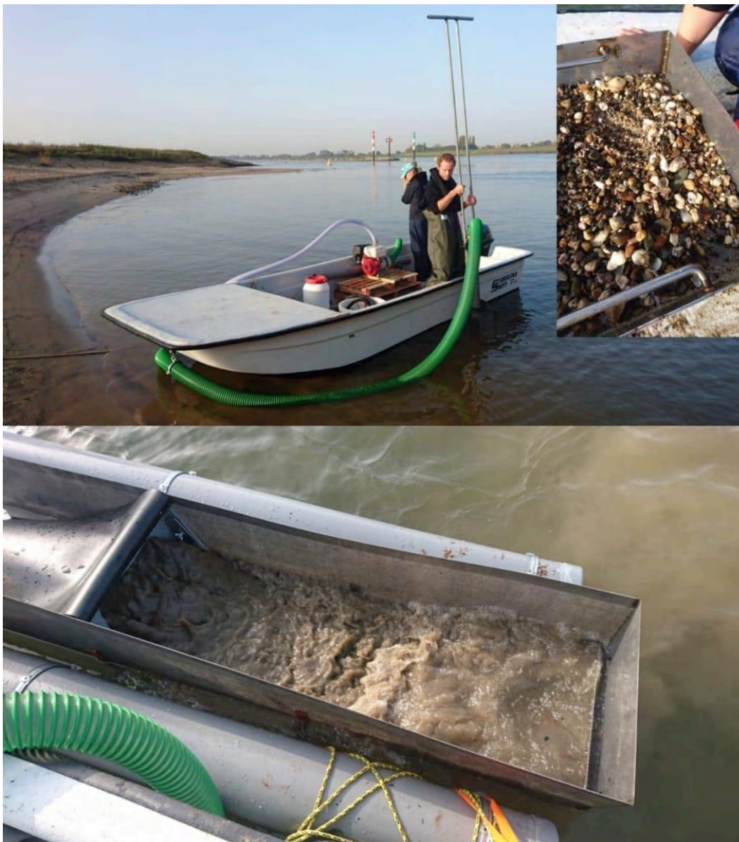
Figure 5 A venturi sediment dredger was used for the sampling of lamprey larvae.
