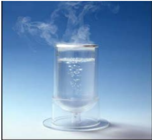
LNG "boiling" at atmospheric pressure and temperature (Source: Osaka Gas Co. Ltd.)
