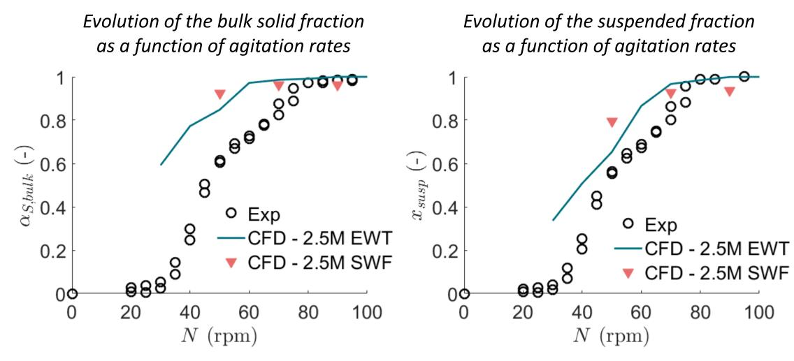
Prediction of a layer without particles up to 90 rpm (not shown)
