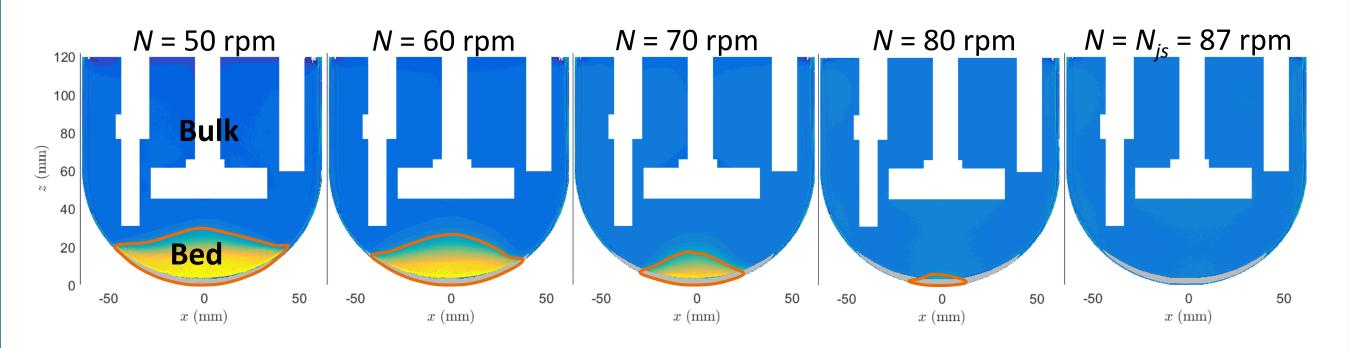
**Bulk:**  $\alpha_{S,bulk} \leq \langle \alpha_S \rangle$  Uniform solid fraction in the bulk at any N
