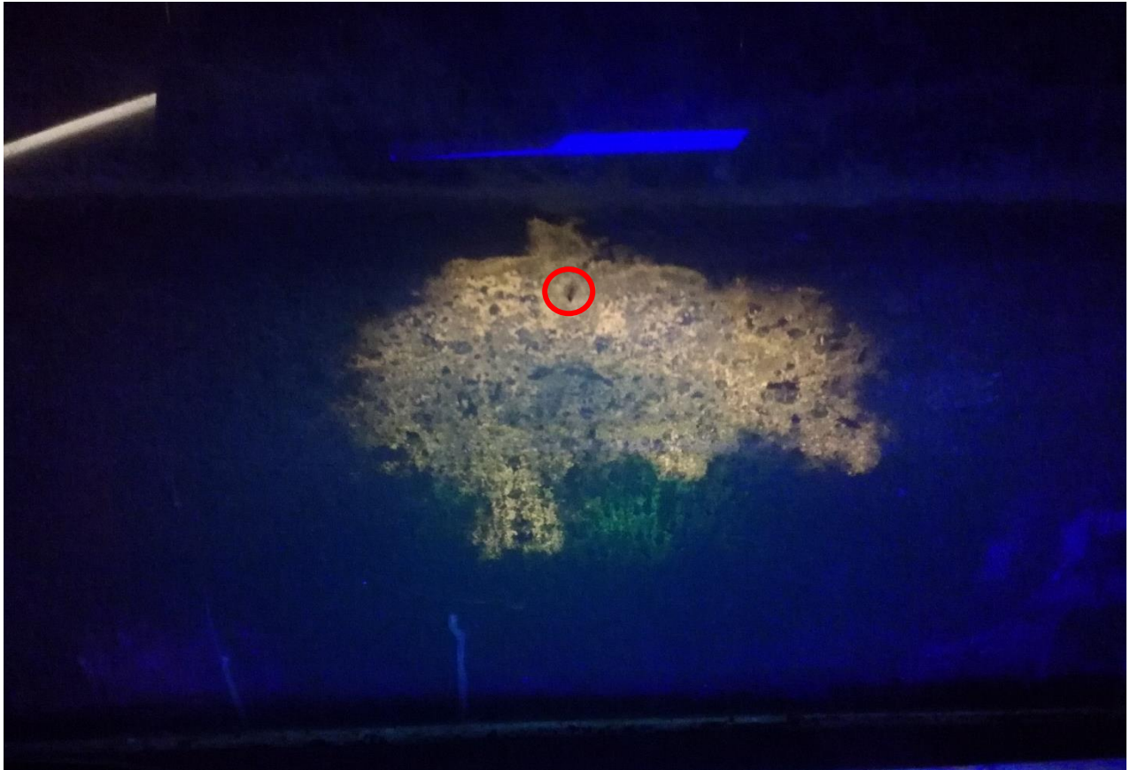
Figure 2.6. The situation after the end of experiment. The maximum width of the contaminated zone was 19 cm and the height was 12 cm. The injection spot is marked with the red circle.
