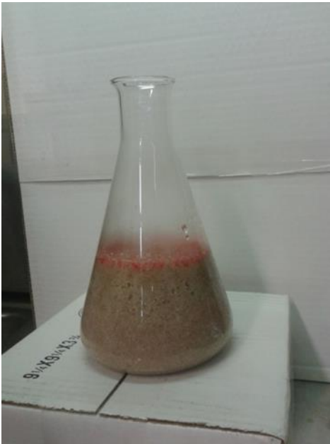
Figure 3.4. Addition of H_2O_2 into quartz sand spiked with red-dyed diesel. The reaction is mobilizing the oil towards the soil surface.
