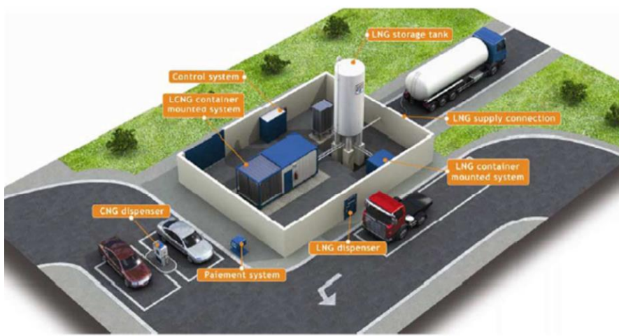
Figure 25. The basic components of an LNG fueling station. Source: [LNG Blue Corridors, 2015] http://lngbc.eu/system/files/deliverable_attachments/LNG%20BC%20D%203.12%20Security%20and%20safety%20issues%20implementation.pdf
