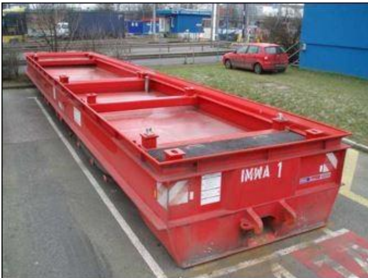
Figure 1: Collection tray for 1x40ft or 2x20ft container. Mobile with coupling on one side and wheels on the other side
