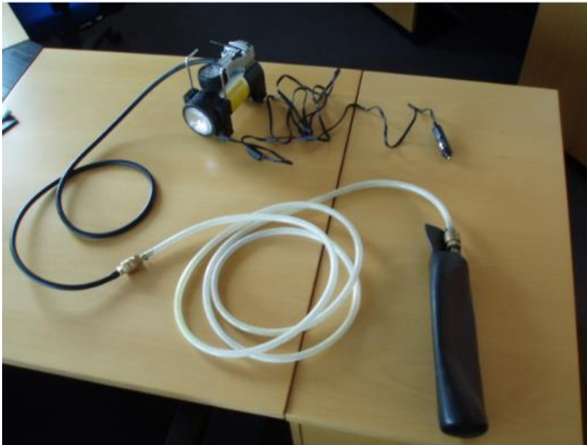
Figure 5: Bladder with compressor for sealing drainage lines
