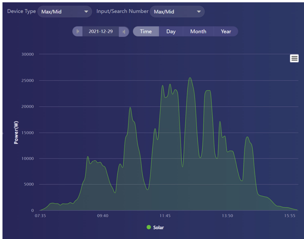
Figure 7.21 Output power of UNISB PV power plant during cloudy day
