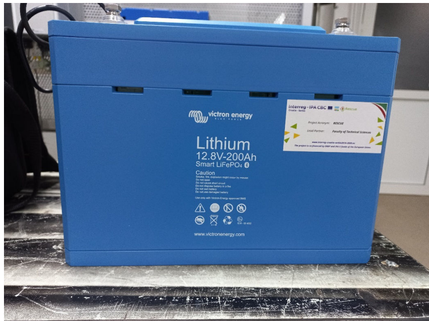
Figure 6.10 Battery within storage-supply system
