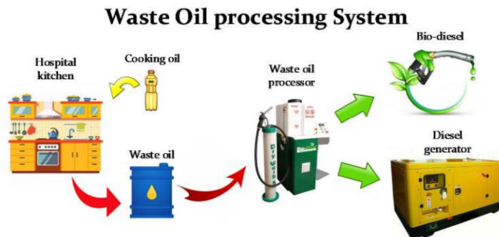
Figure 5.39 Principal schematic of system for biodiesel production from waste oil
