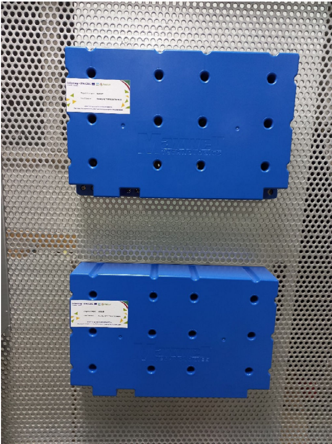
Figure 6.9 Supercapacitors within storage-supply system
