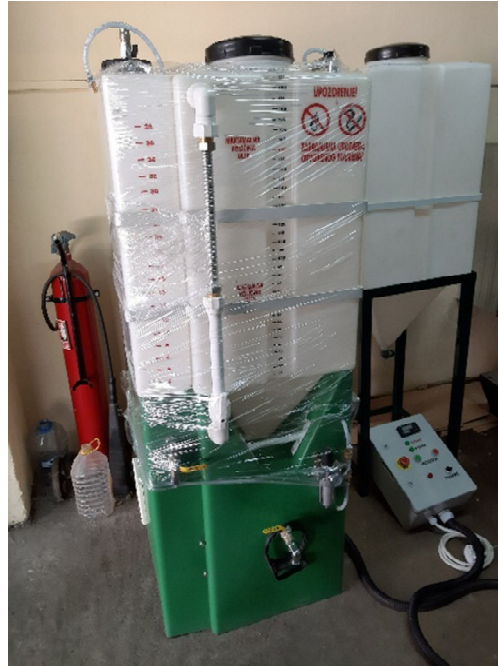
Figure 6.40 KBCO biodiesel production system from waste oil
