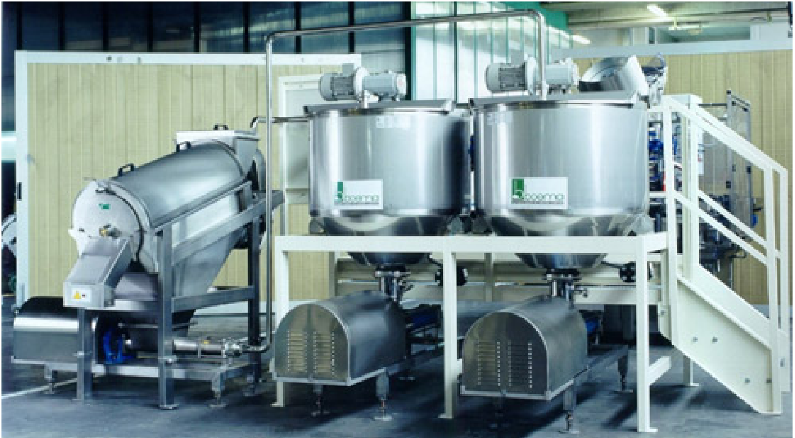
Puree refining and extraction unit Line capacity: up to 600 Kg/H.
