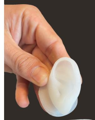
Pam technology makes it **possible to process highly flexible materials**, unlike conventional FDM, SLS and SLA processes.
