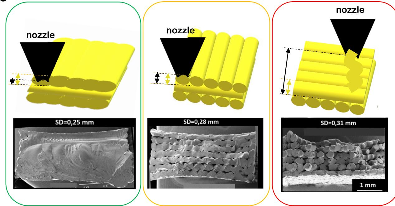
Contact bead =  $f(\text{process parameters})$
