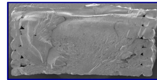
Challenge: Control of the level of porosity → mechanical properties
