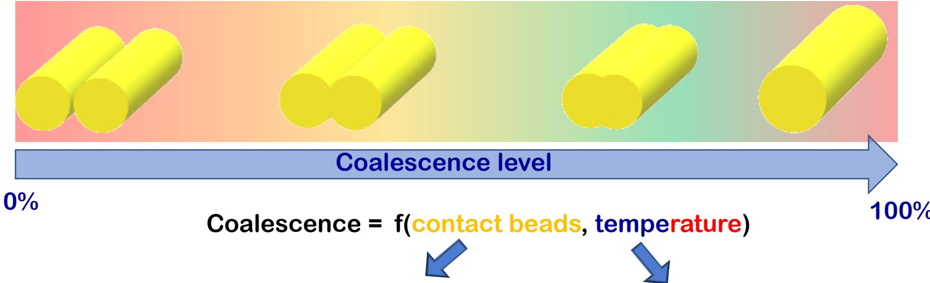
Contact bead = f(process parameters)
