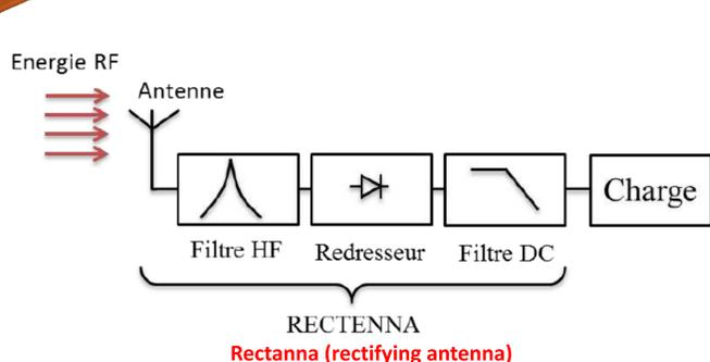
The Schottky diode is the main part of the Rectenna in order to rectify the input AC signal and deliver the DC output signal required to power the main circuit.
