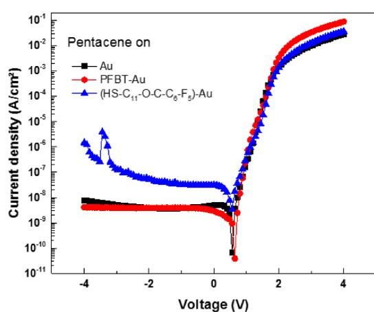
DC current density-voltage characteristics for pentacene and Polyera N200 diodes with and without SAM coating on the Au anode.
