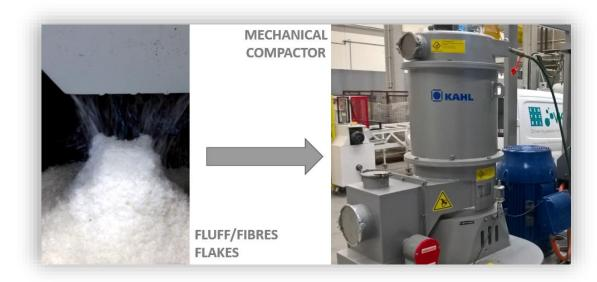
As polyester is involved, the pellets must be crystallized before thermo-granulation, and they must be dried.
