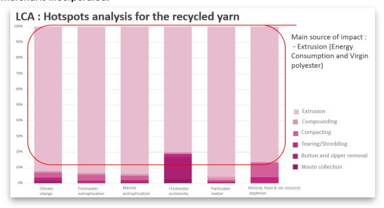
If we look at the detail of the impacts per stage of this value chain, we can see that on all the indicators, it is the extrusion phase that represents 80 to more than 90% of the impact. This is mainly due to the energy consumed in extrusion and the addition of 50% virgin polyester.
