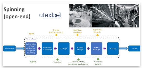
Finally, the open-end spinning at Utexbel, with mainly material preparation, carding and spinning + winding to obtain the 30/1 yarn.
