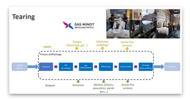
The fraying process is then broken down mainly into a cutting stage of the unraveled textiles, a mixture, the actual fraying (i.e., to return to the fibre) and the press to create bales of fibre. The
