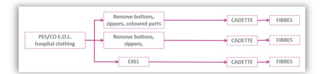
After extensive discussions with all partners in the value chain, it was decided, especially at the request of the spinner, to remove all hard parts (buttons, zips, etc.) in advance in a separate process step
