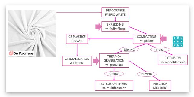
Monitoring of the intrinsic viscosity value throughout the process shows that there is a significant decrease in intrinsic viscosity during compaction and thermogranulation, which, without intervention on the material, will cause a significant embrittlement of the material once extruded and a poorer processing during extrusion.
