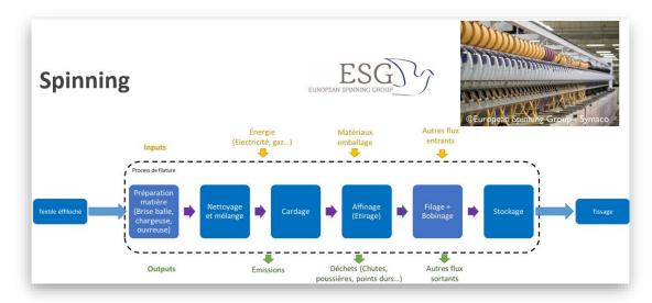
For the spinning phase, ESG has carried out this stage for this value chain. The spinning process is classical, with a preparation of the material, a carding stage before spinning the yarn.
