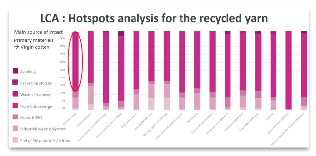
If we look at the details of the recycled yarn, we can see that **70% of the impact comes from the added virgin cotton (which is a known polluting material).** One possibility to improve the environmental balance of the product would be to integrate recycled cotton fibre.
