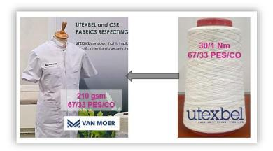
Throughout the process, the used garment, which originally contained 65% polyester and 35% cotton, lost 25% of the cotton fraction at the carding tape stage with a composition of 90% polyester and 10% cotton. The spinner therefore added virgin material for a viable recipe: a 1/30 Nm Open End yarn with 35% virgin cotton, 65% Polyester (25 frayed, 25 production off-cuts and 15 RPET bottles) and then a 210 a/m2 fabric.
