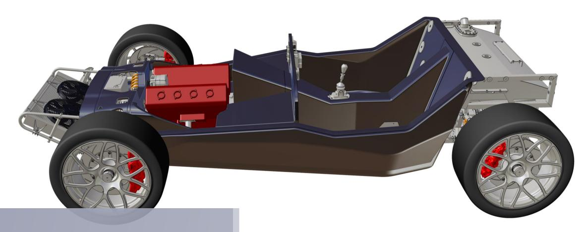
Chassis Nomex / Carbon fiber mono-shell
