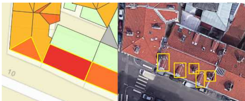
Figure 2: Illustration of constraints induced by superstructure elements
