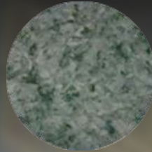
Shredded bag of PLA + PBAT based Biopolymer (BP3)
