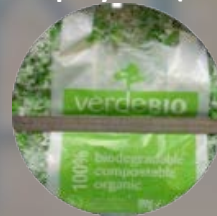
Shredded bag of PLA + PBAT based Biopolymer (BP3)
