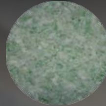
Shredded bag of PLA + PBAT based Biopolymer (BP4)
