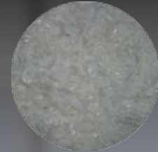
Shredded bag of PE with oxo degradable additive (OXO)
