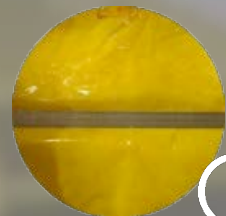
Shredded bag of PE with oxo degradable additive (OXO)
