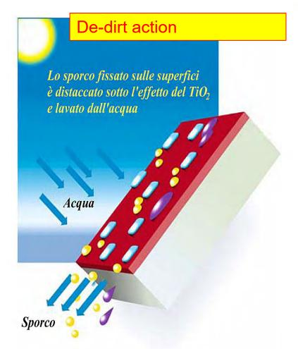
Under the action of UV rays, the particles of TiO<sub>2</sub> transform organic compounds, odors and BACTERIA, close to its surface in water and carbon dioxide.
