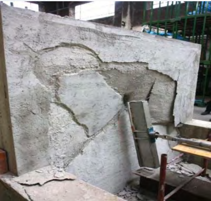
Partition wall with force on the side with Aegis in cement plaster.
