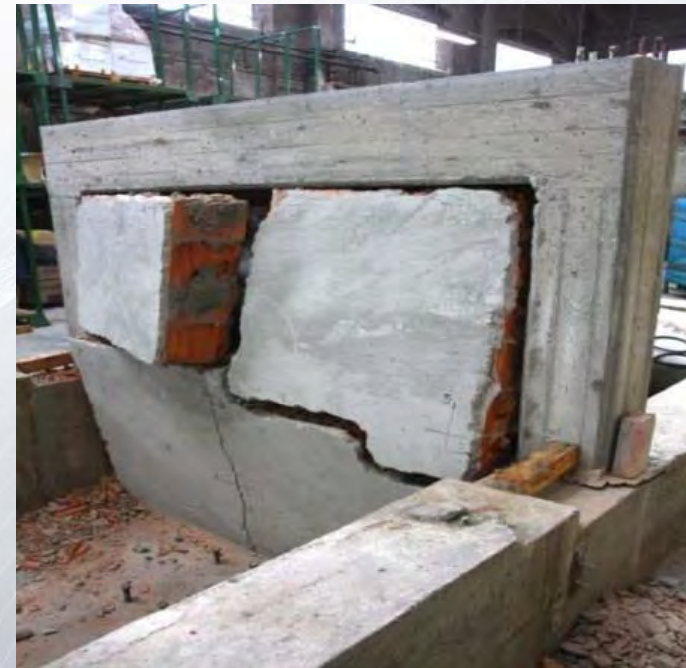
Side opposite to Aegis, no contact with columns or beams. Breakage but no falling of wall parts
