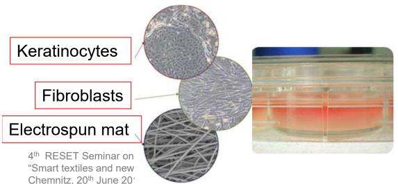
The product generated in this project consists of a electrospun scaffold combined with a dermal equivalent made of fibroblasts and keratinocytes:
