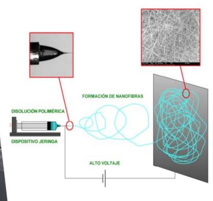
**Polymers for bio-responsive** applications and biomedicine must be selected from 'medical grades'. Here we focus on the treatment of severe burn injuries using electrospun mats (monoaxial) of bio-compatible poly(D,Llactide-co-glycolide) (DLPLG).
