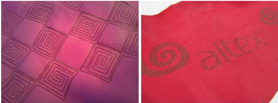
Decoration of natural leather using laser marking
