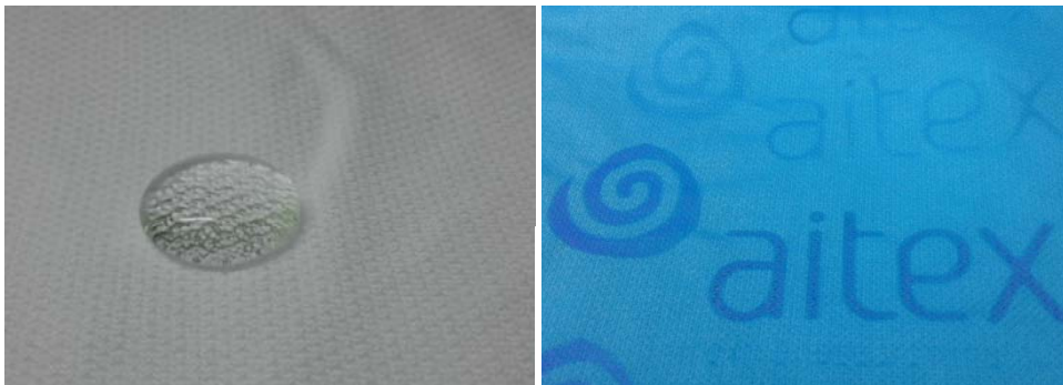
Left) PES fabric finished via nanobubbles; right) PES t-shirt marked with laser
