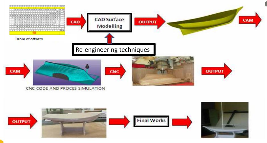
Illustration of main steps for the production of wooden model Table of offset- 3D Modelling – CAM Processing – CNC –Final Product
