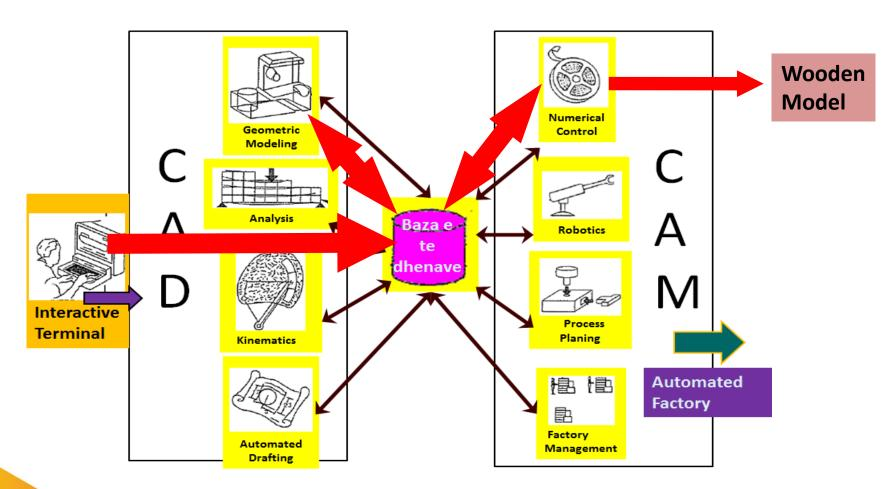
Main organisation structure of a CAD/CAM System used in an automated factory (adapted from Ship Production, 1995)
