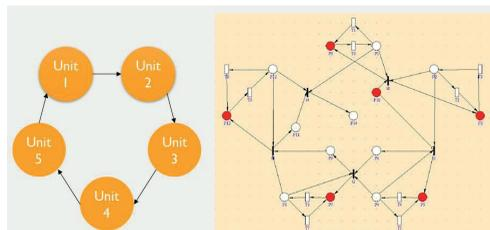
Figure 10. Petri net which models mutual testing for system with five units.
