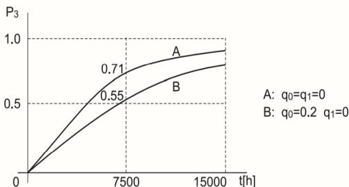
Figure 2. Probability of system failure,  $P_3(t)$ .
