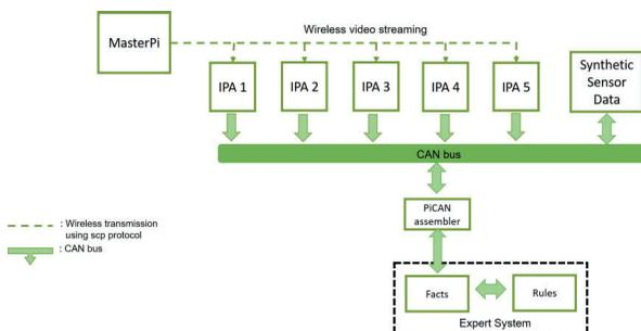
Figure 1: Communication System for the Raspberry Pi's.
