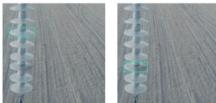
Fig 6 shows an example of a false positive on the left image as the bounding box is surrounding a functional insulator and a true positive on the right in which the discolored insulator is detected and bounded by a box.
