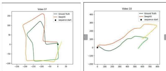
Fig.1. Visual Odometry generated for deep VO for trained model over dataset
