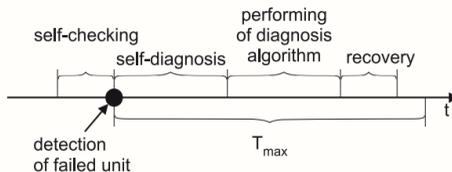
Figure 5. Duration of procedures which provide system fault-tolerance.
