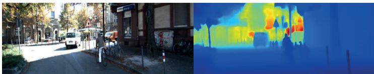
Fig 5. left: RGB image KITTI dataset. Right: Corresponding depth image using Jet colormap, the shorter distance object to the camera, colormap represent blue, the farthest object, the colormap represents red and object between short and farthest distance object represents green
