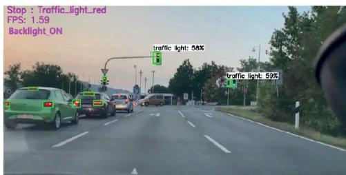
Figure 6: Traffic Light and Backlight Detection
