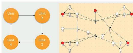
Figure 11. Petri net which models mutual testing in the system after removing faulty unit.
