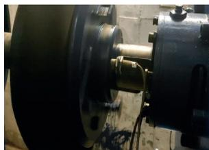
Induction sensor for RPM measuring
