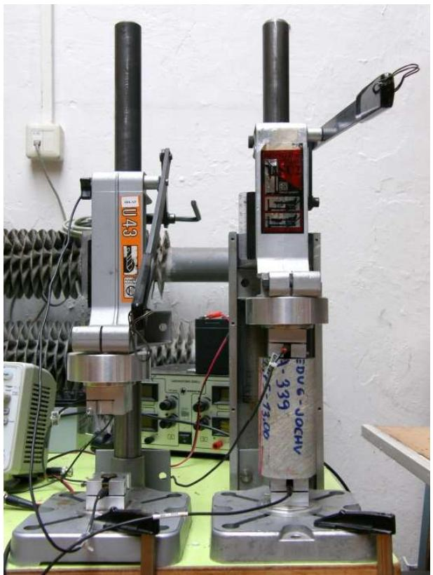
$$E_d = \frac{\rho v_s^2 (3v_p^2 - 4v_s^2)}{v_p^2 - v_s^2} \quad v_d = \frac{v_p^2 - 2v_s^2}{2(v_p^2 - v_s^2)}$$
