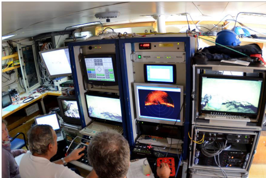
The control room of ROV Max Rover on R/V AEGAEO.
