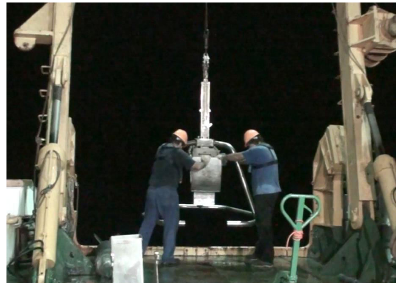
Box corer deployed through the A frame at the stern of R/V Aegaeo
