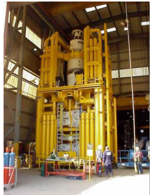
Subsea BOP stack
