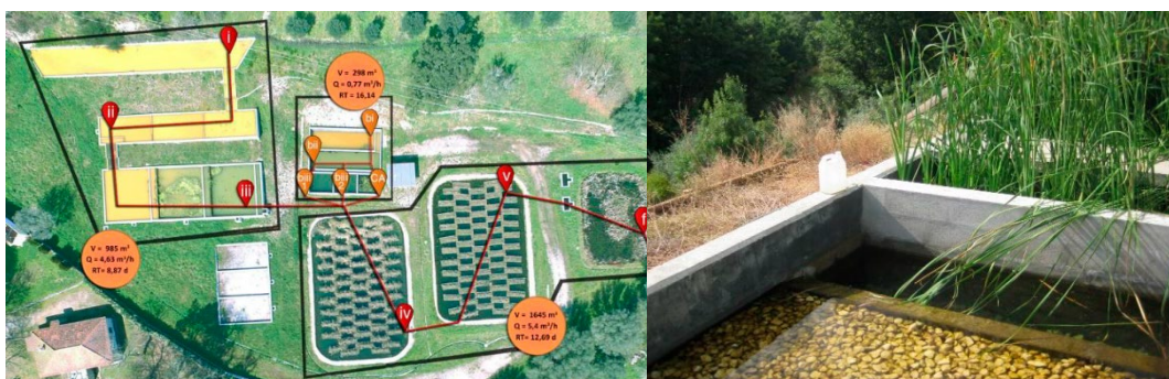
Figure 10 - Urgeiriça (shaft n.º 4) mine water passive treatment system layout and hydraulic data (V= Volume; Q= Flow; RT = Retention time) (Pinto et al., 2015)
