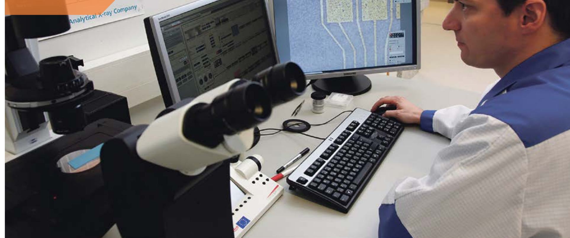
Laboratory professional is inspecting a ceramic electronics substrate with inverted research microscope.
