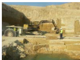
Extraction of blocks of Villamayor sandstone
