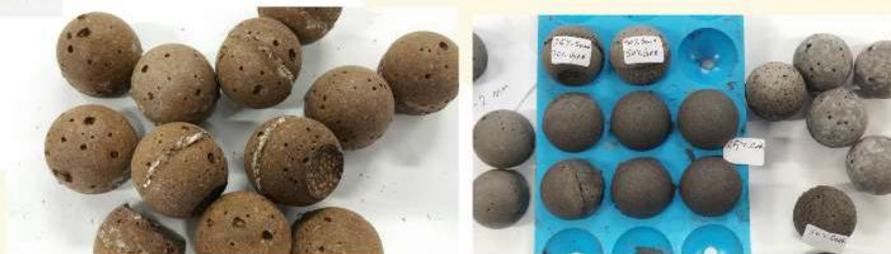
lightweight foamed materials, combining mud + waste glass + expanded cork
