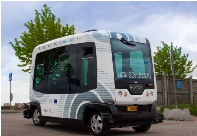
Picture: SOHJOA-pilot project is testing autonomous electric in nordic street environment.
