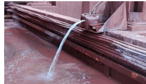
Filtrate is returned to washers, and re-introduced to the Bayer cycle
