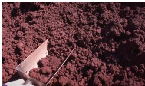
Bauxite Residue discharged with moisture between 26-28%
