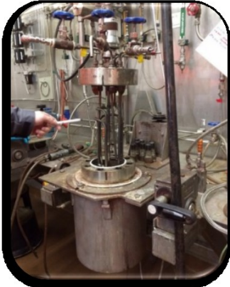
Pressure leaching reactor (autoclave)
