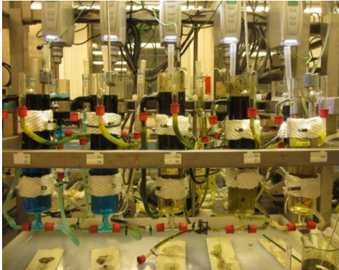
Cu-Zn SX small scale pilot plant
