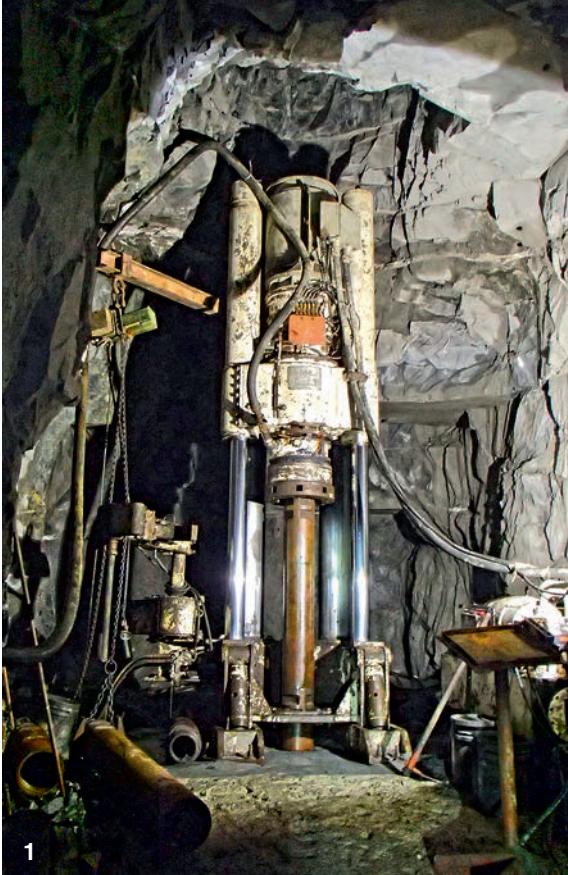
Mine operations: (1) Raise-borer; (2) Low profile loader; and (3) Jumbo.
