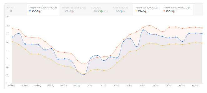
Fig.21. One month temperature evolution in 3 rooms of an apartment
