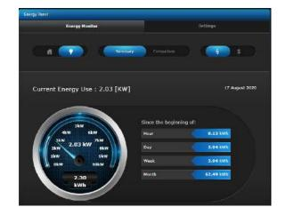
*Fig.16. Energy panel shows instant power and electricity consumption (hour, day, week, month)*
