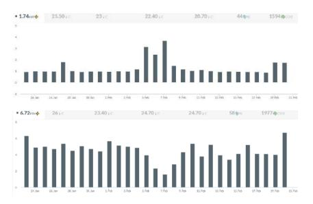
Fig.4. Daily electricity consumption for one month, apartments D and H
