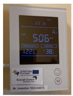
Fig. 10. Climate unit displays CO2, temperature, humidity and qualitative info for VOC
