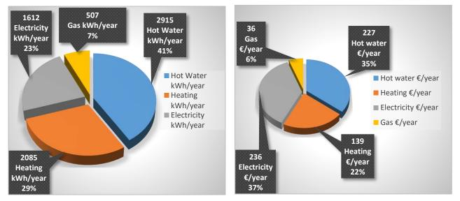
Fig.18. Average energy consumption/apartment/year Fig.19. Average energy cost/apartment/year
