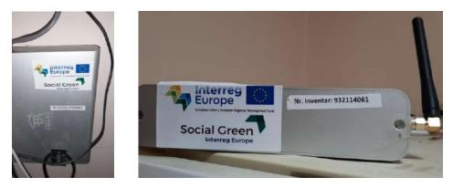
Fig.2. Smart Home Gateway – in 2 configurations, connected to internet using Ethernet cable; antenna is for Z-Wave communication with sensors
