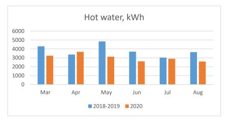
Fig.32. Monthly energy consumed for hot water in all social apartments, kWh, before and during project
