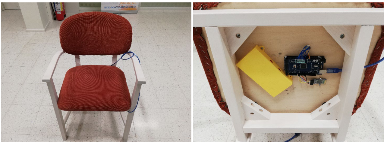
An ordinary chair with armrests was used for installation of the pressure sensors (left photo). Bottom of the chair showing connectivity to the pressure sensors within the cushioning and a power bank (right photo).
