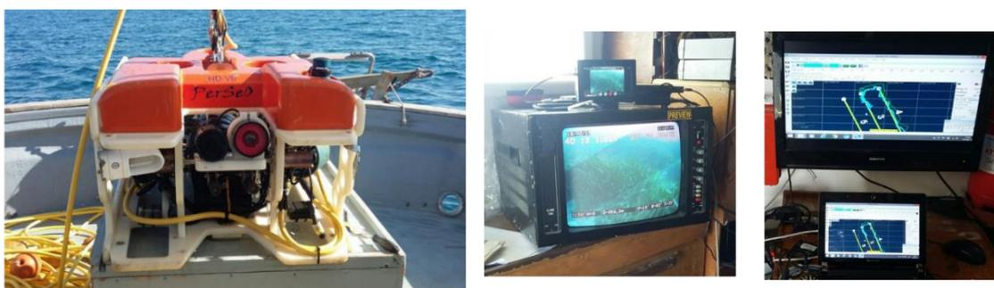
Figure 25, ROV Equipment used during the coralligenous survey at Torre Guaceto and Porto Cesareo.
