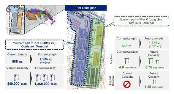
The port's Master Plan was developed in alignment with ThPA SA strategic directions, as well as the predictions made for its throughput up to 2040. The investment plan includes the expansion of pier 6 (container and dry bulk), in order to serve vessels of more than 8000 TEU, thus increasing its capacity.
