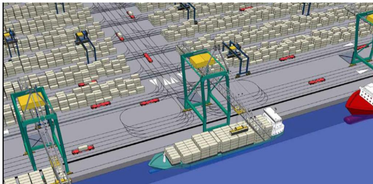
Fig. 2: Operative scheme with AGVs
