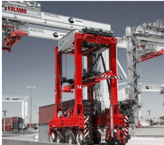
Figure 23: Automated Straddle Carrier
