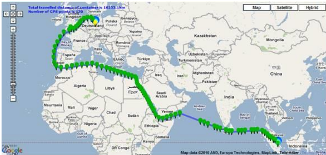
Figure 14. The Schenker Smartbox real time tracking ICT (Source: Zacharioudakis et al., 2012)
