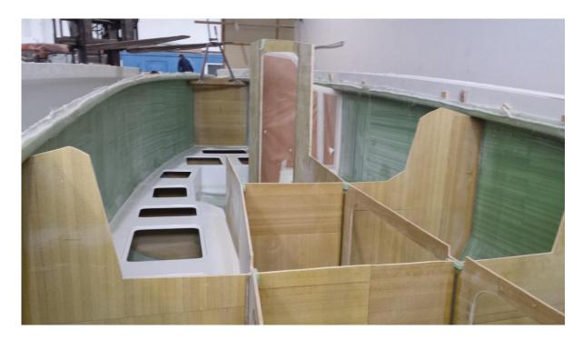
Internals: for the corporate (mixed crew) use a real standing height bathroom with fixed shower, wash bassin and marine head was a non negotiable must, so we positioned it on Starboard side of the keel box, that thanks to the reverse sheer and chined hull offers a lot of volume despite the limited beam – the result is really impressive for a boat of this size. A front V berth/dinette, a central mini galley on Port and two symmetric aft berths round up the accommodation.
