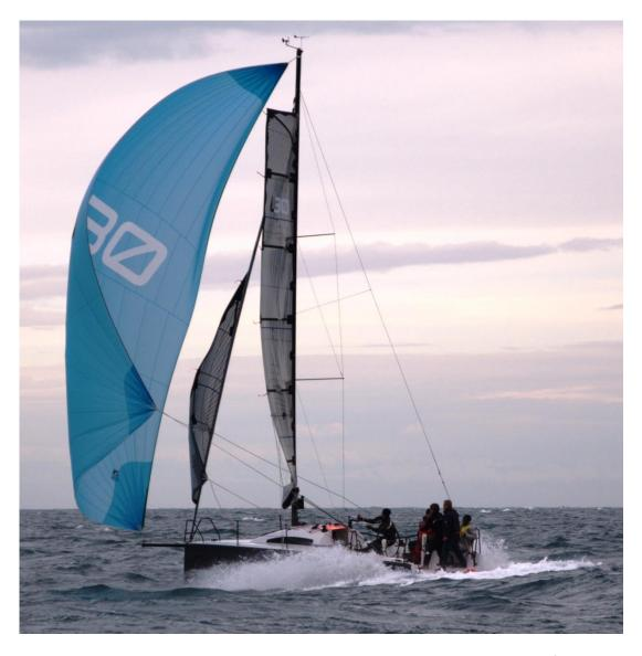
Despite the good VPP numbers, we were a bit concerned about the low wind performance and we were considering a taller mast option as a back up plan. But already on the second trial day, with 4-6knt of TWS, we were sure there is no need for more power, the hull is really easy to drive.
