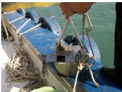
Picture 2.8: Sediment sample is collected from the seabed using a special grab
