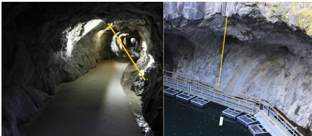
Figure 10.6. Examples of in-situ measurement using portable rangefinder in underground workings (left) and overhanging roof (right)
