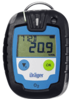
Figure 6.17. Portable oxygen detector DRÄGER PAC 6000 ( www.draeger.com )
