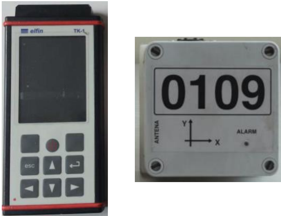
Figure 6.8. Inclino-metric measurement system: communication terminal (left) and a CNS sensor (right) (Stolecki & Grzebyk, 2014)
