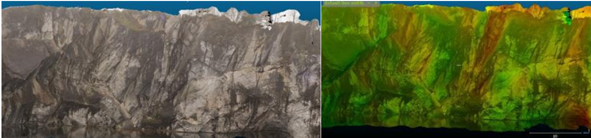
Figure 10.1. The stability of the vaults in the walls of the Ruskeala quarry in the original survey (left) comparison of changes after a year (right)
