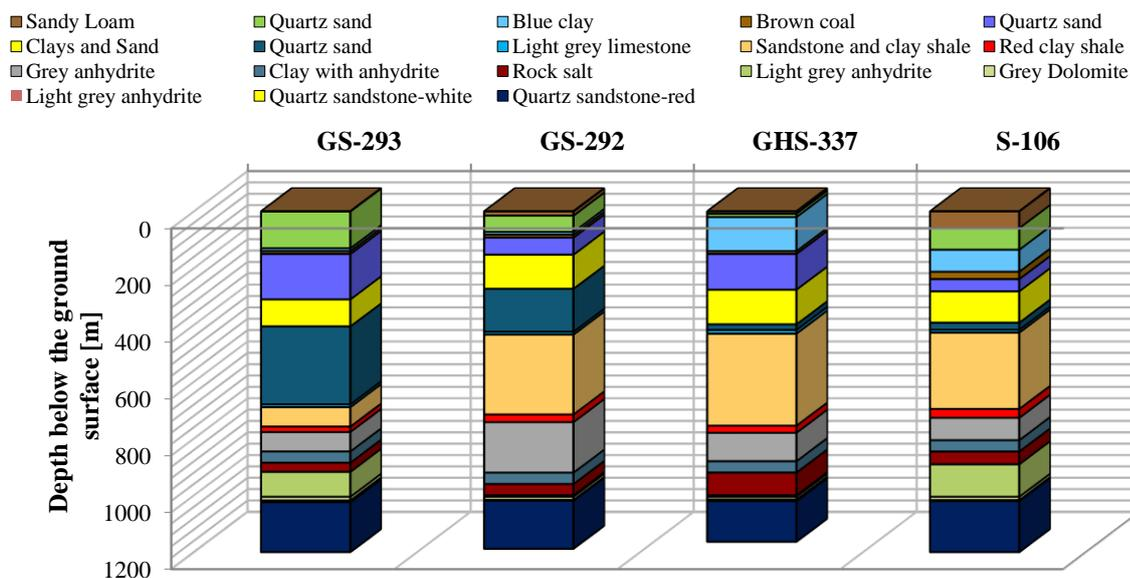
Figure 4.17. The layering of strata in analyzed boreholes
