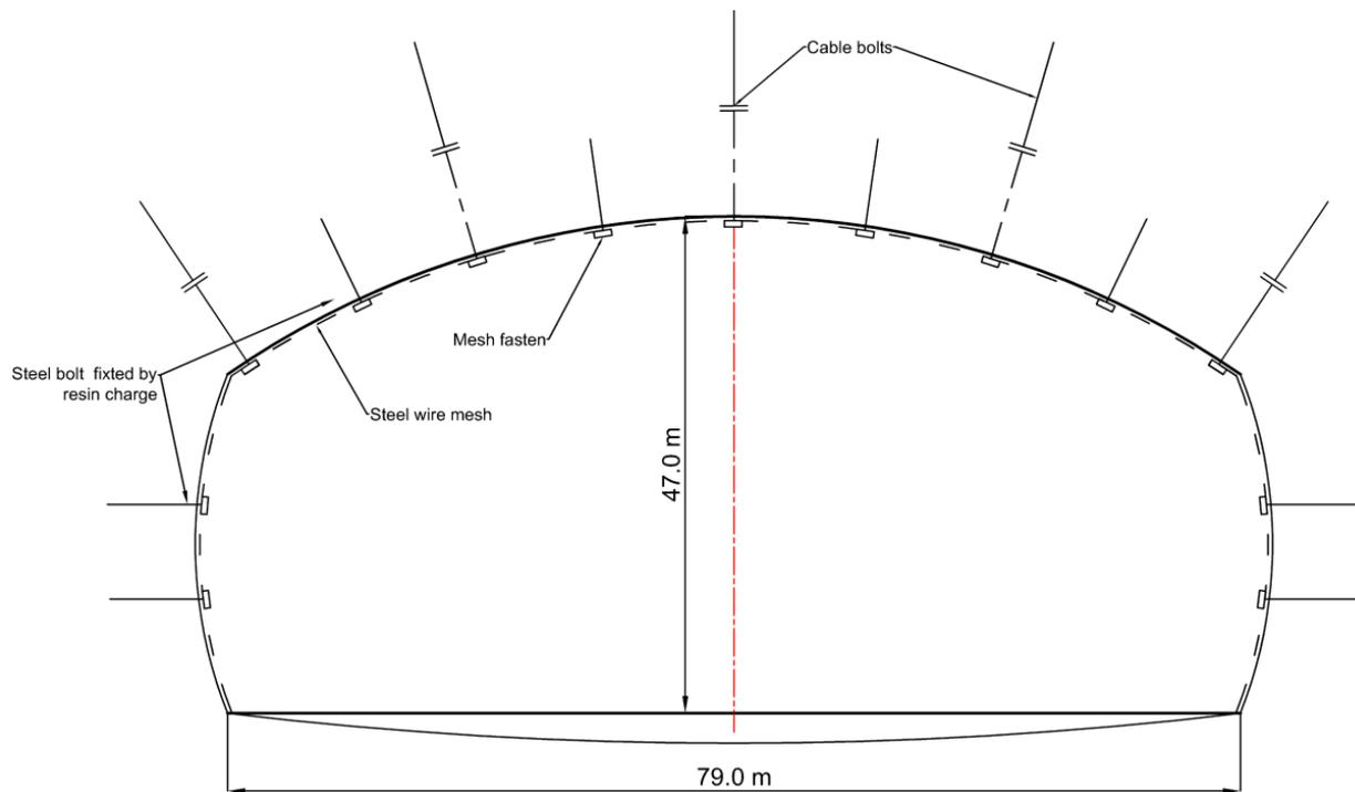
Figure 4.4. The dimension of the main laboratory chamber
