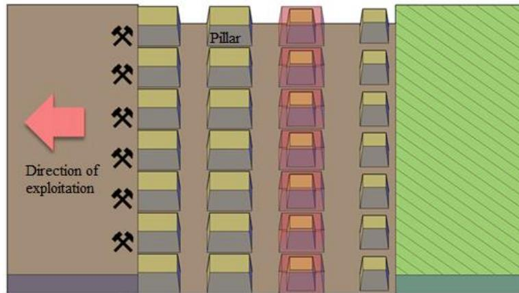
Figure 3.2. The basic scheme of Room-and-Pillar mining method
