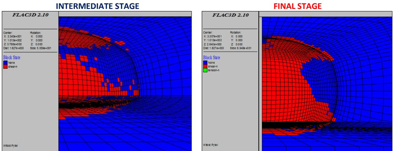
Figure 4.8. Spalling of chamber surface – location of the yielding (unstable) blocks (x-z cross-section)
