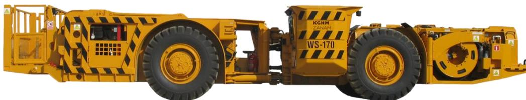
Figure 3.19. An example of a bulk emulsion production unit (KGHM Zanam, 2020)
