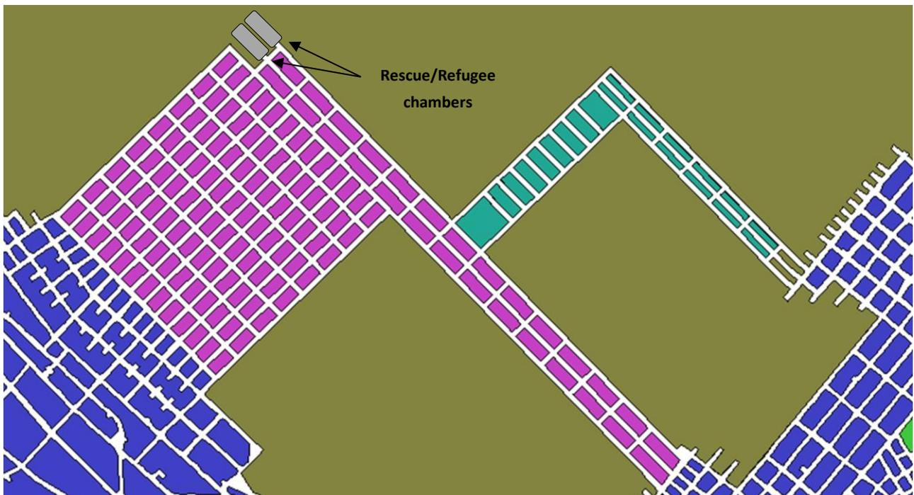
Figure 6.14. Location of safety chambers in vicinity of the front line of trial mining poanel
