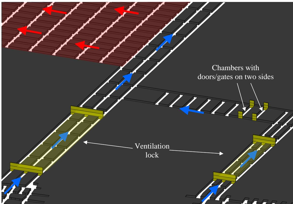
Figure 6.13. Scheme of air distribution through projected trial mining panel and location of ventilation locks
