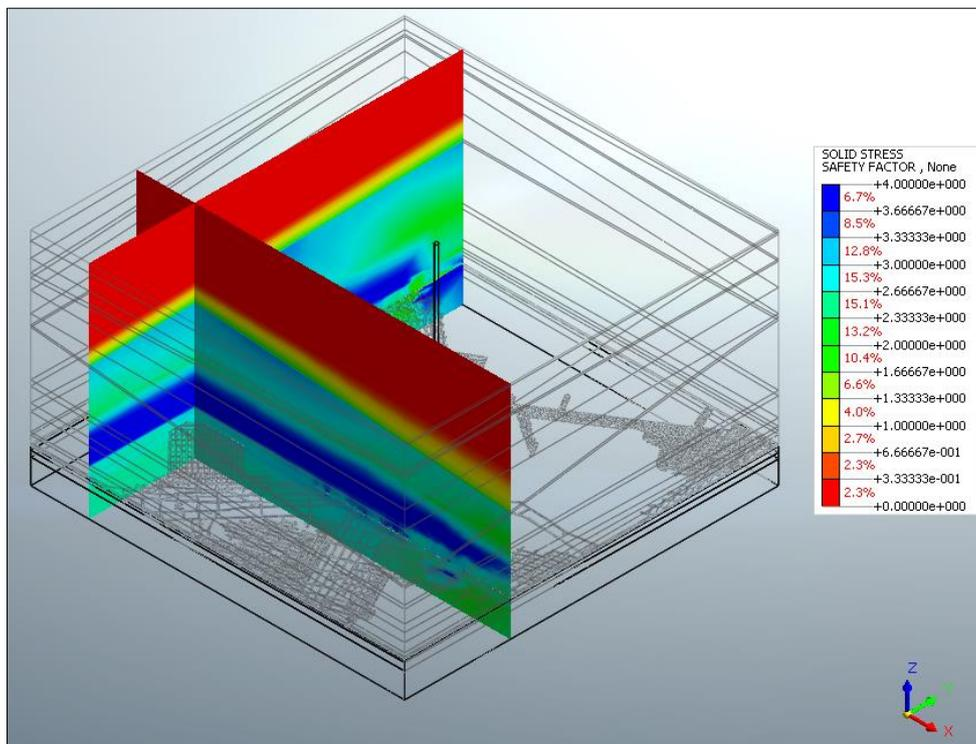
Figure 4.27. Verticals through the base of the trial panel (horizontal) and boundaries of a numerical model (vertical)
