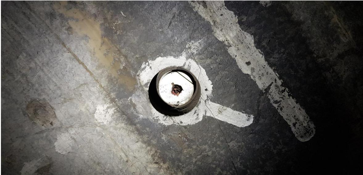
Figure 6.11. Device for Crack detection signaling
