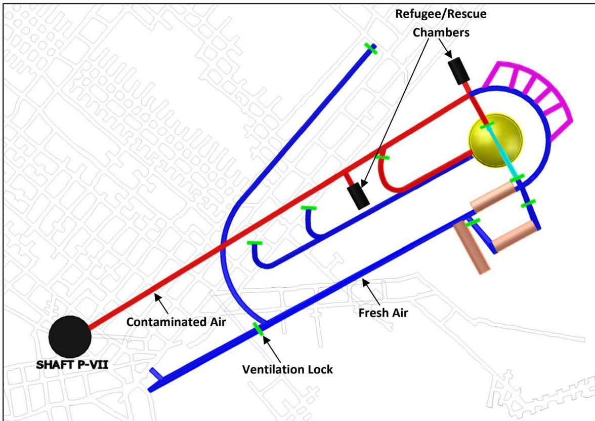
Figure 6.4. Scheme of air distribution through projected workings and location of ventilation locks
