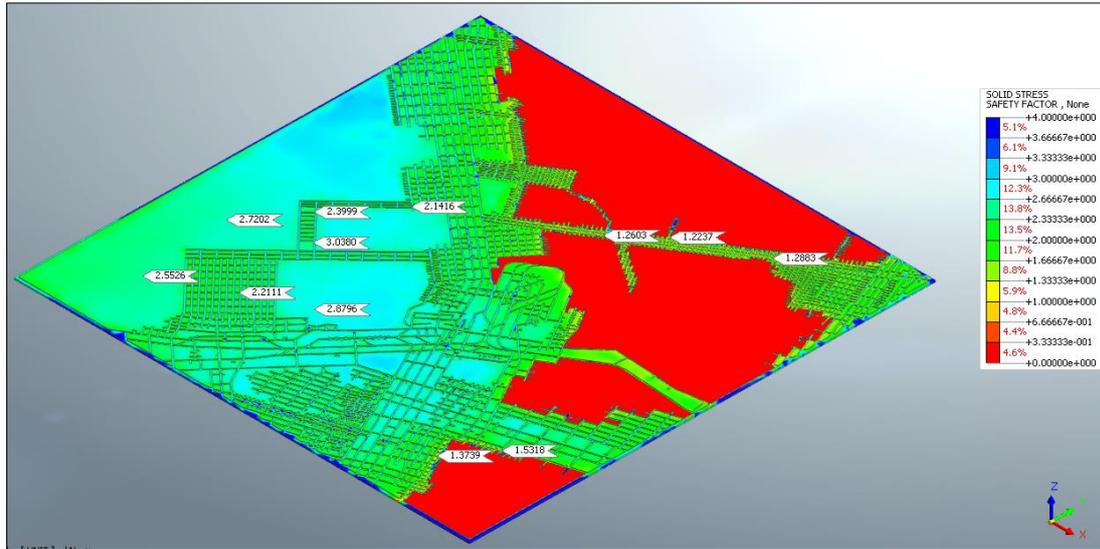
Figure 4.24. Contours of SF values at the level of conceptual mining panel
