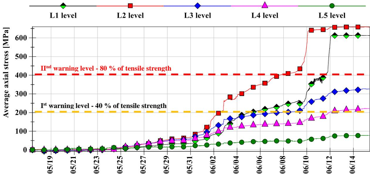
Figure 6.2. The principle of roof fall hazard warning with the use of instrumented rockbolts
