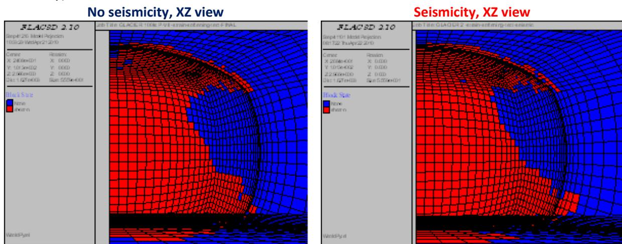
Figure 4.9. Selected results of calculations - spalling of the chamber (x-z cross-section)
