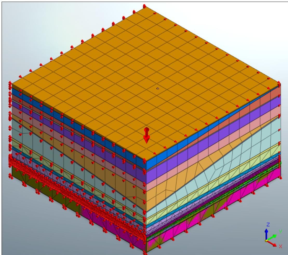
Figure 4.20. The external geometry with mesh and boundary conditions of the 3D UL model
