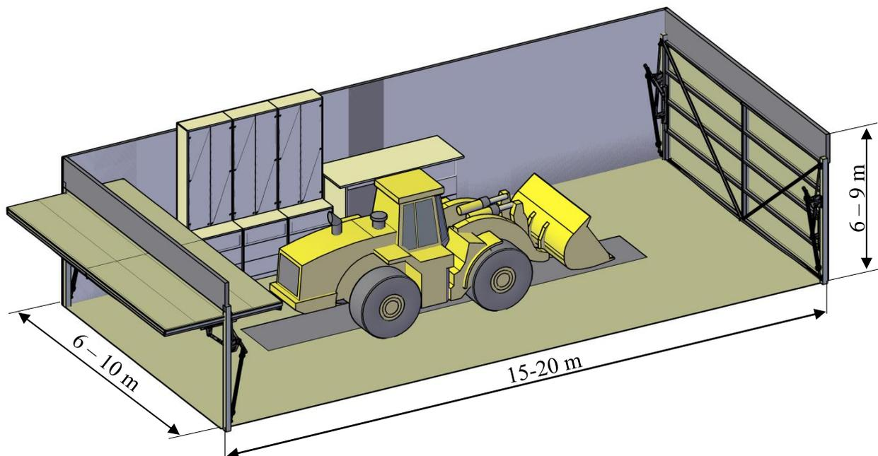
Figure 6.6. Conceptual shape and arrangement of a machine chamber located near the trial mining panel
