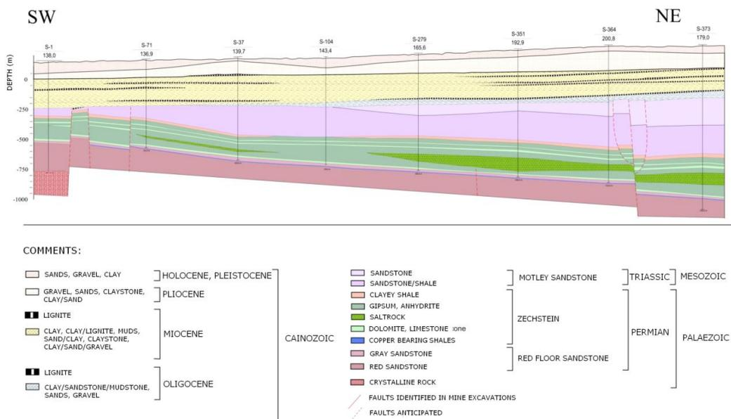
Figure 3.5. Geologic cross-section in Polkowice-Sieroszowice mine
