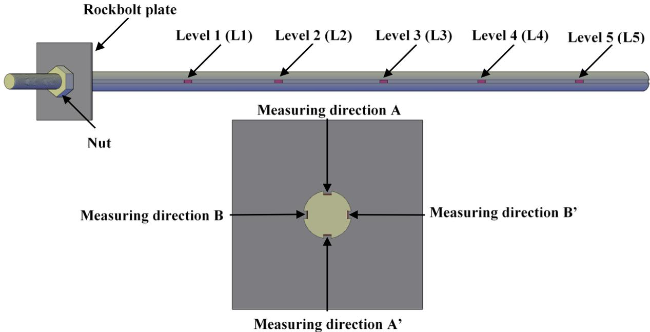
Figure 6.1. Scheme of instrumented rockbolt for continuous stress, strain measurements
