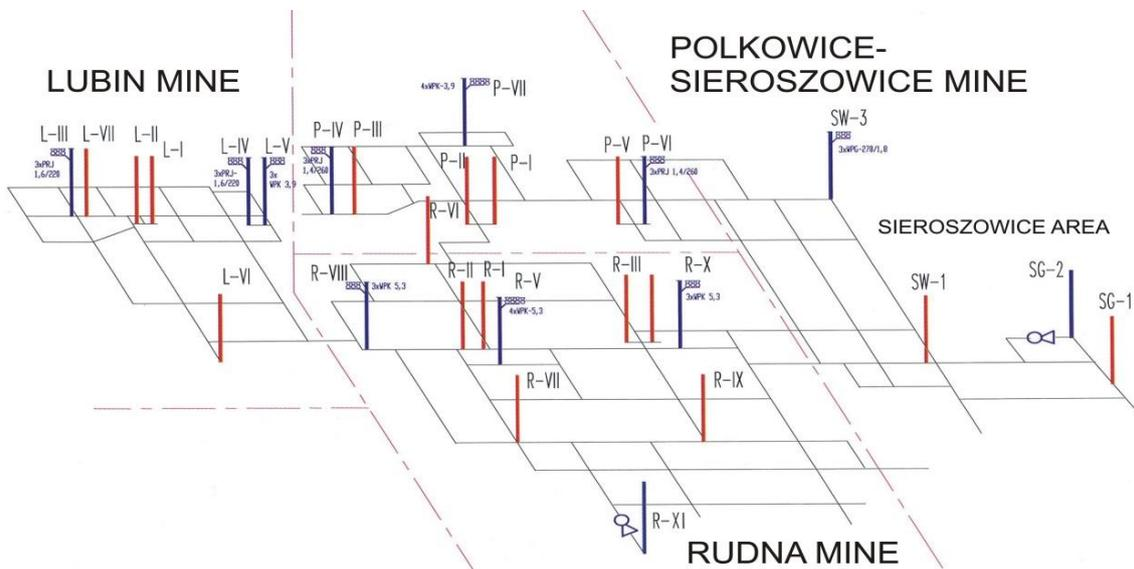
Figure 3.12. Simplified scheme of the ventilation system in KGHM mines
