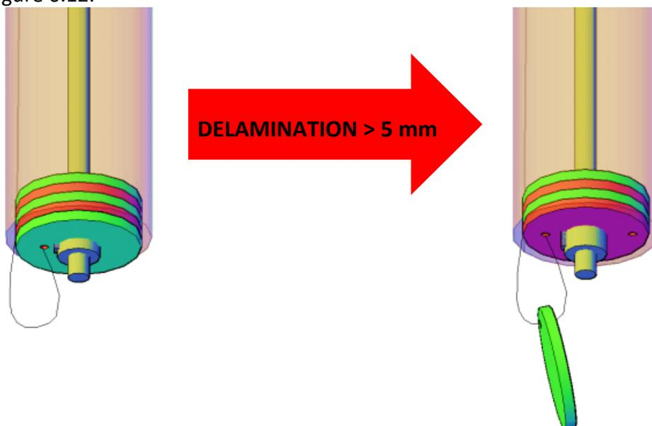
Figure 6.12. The principle of roof delamination warning
