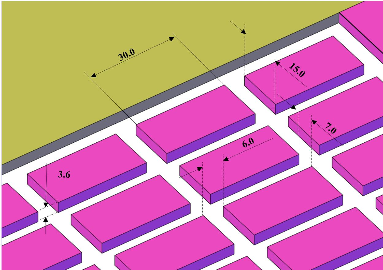
**Figure 4.14. The geometry of pillars and working within the projected trial mining panel**
