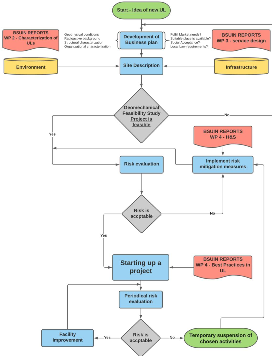
Figure 8.1. Flowchart representing the process of sustainable UL development
