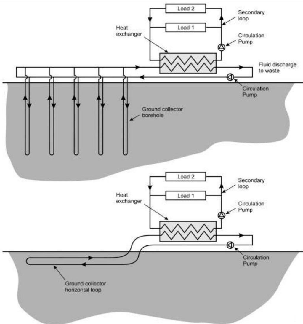
Fig. 1 B. Conceptual sections through a closed loop geothermal system. After Preene & Younger (2014).
