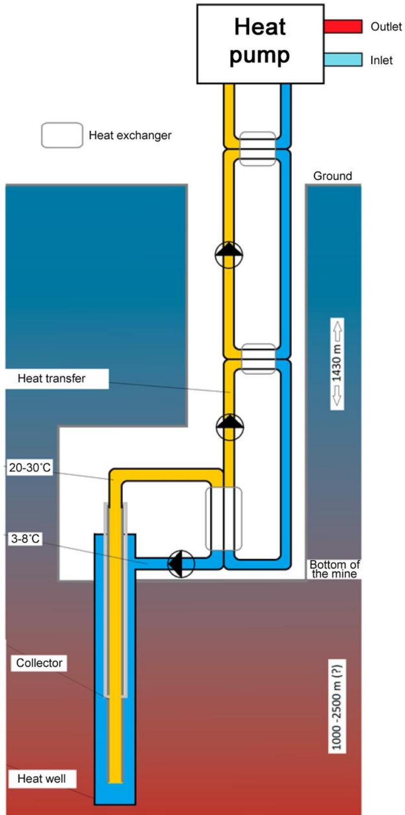
Fig 4. A conceptual model for the proposed geothermal energy production in the Pyhäsalmi mine. Modified from Ahonen et al. (2020).
