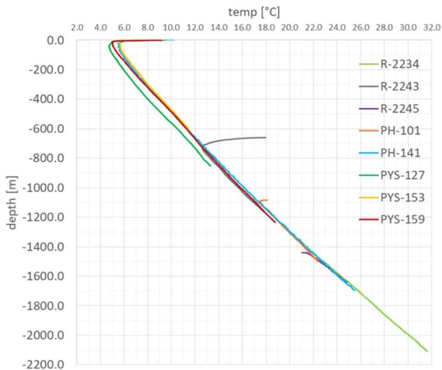
Fig. 3. Temperatures in the bedrock as measured from different boreholes by a DTS cable.
