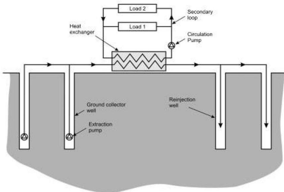
Fig. 1 A. Conceptual sections through an open loop geothermal system. After Preene & Younger (2014).
