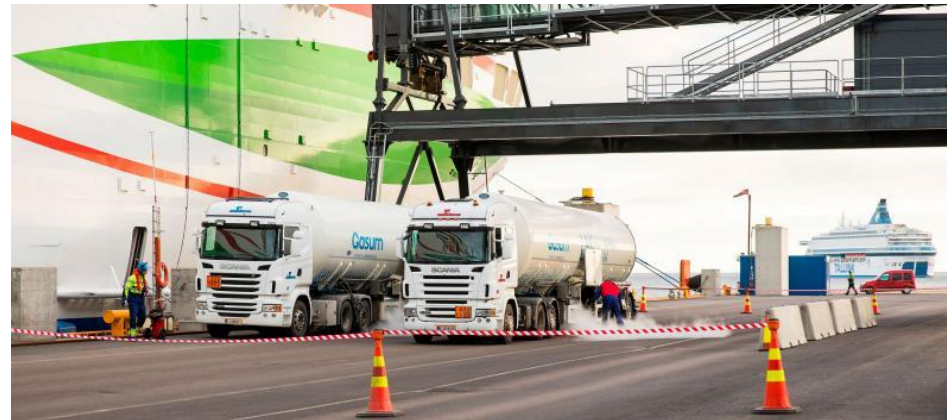
Ref: https://www.portofhelsinki.fi Truck-to-ship LNG bunkering at the Port of Helsinki
